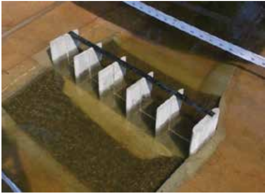
Figure 1 - Fixed Bed Model with Proposed Salinity Barrier (for Nilwala River)
