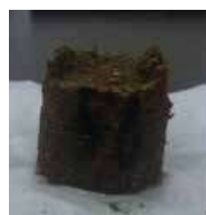
50% sawdust 50% rice husk briquette after water permeability test
