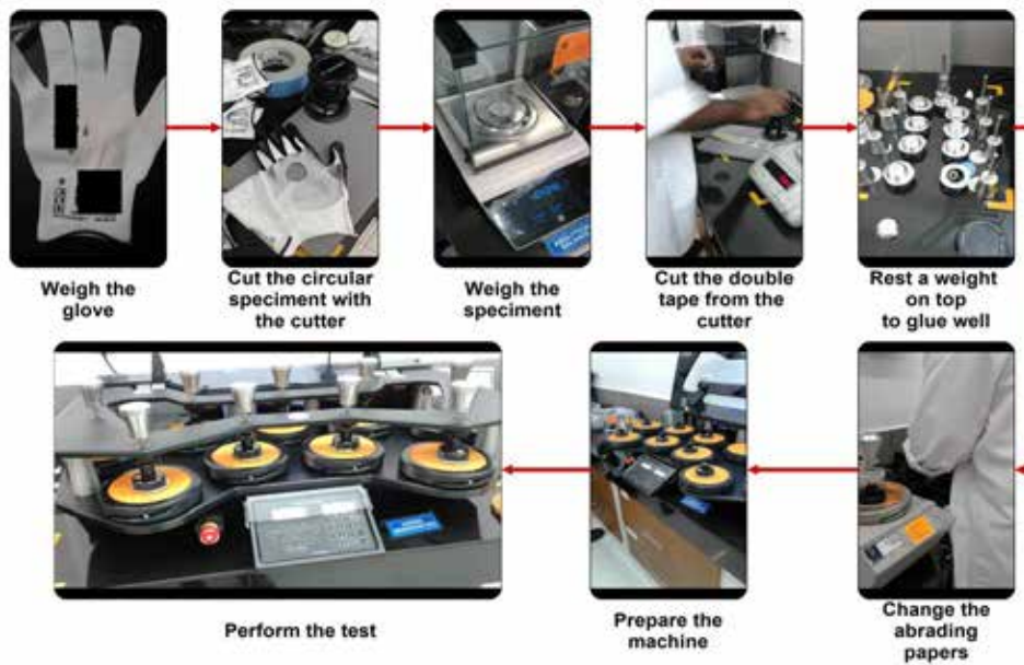
Figure 2 – Abrasion resistance testing process
