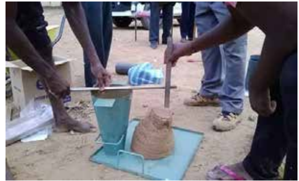
Figure 2 - Measuring slump of backfill
