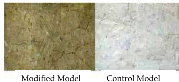
Figure 2 - Crack patterns in two soil models [4]
