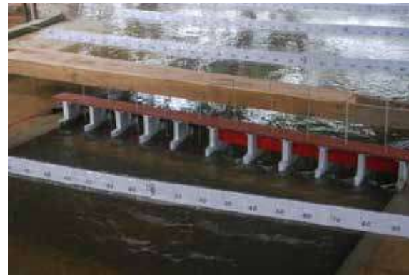
Figure 8 - Simulation of Flood Condition with partial gate opening condition
