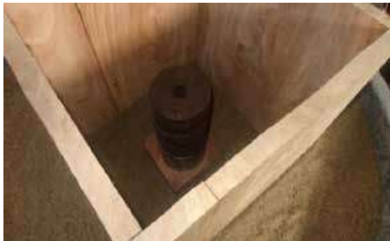
Figure 5 - Placing the steel plate loads
