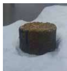
100% sawdust briquette after water permeability test
