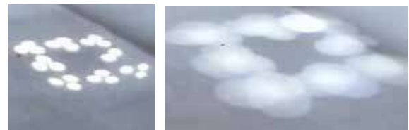
(a) (b) Figure 17 - Light patterns at the receiver (a) Focused, (b) Not focused.
