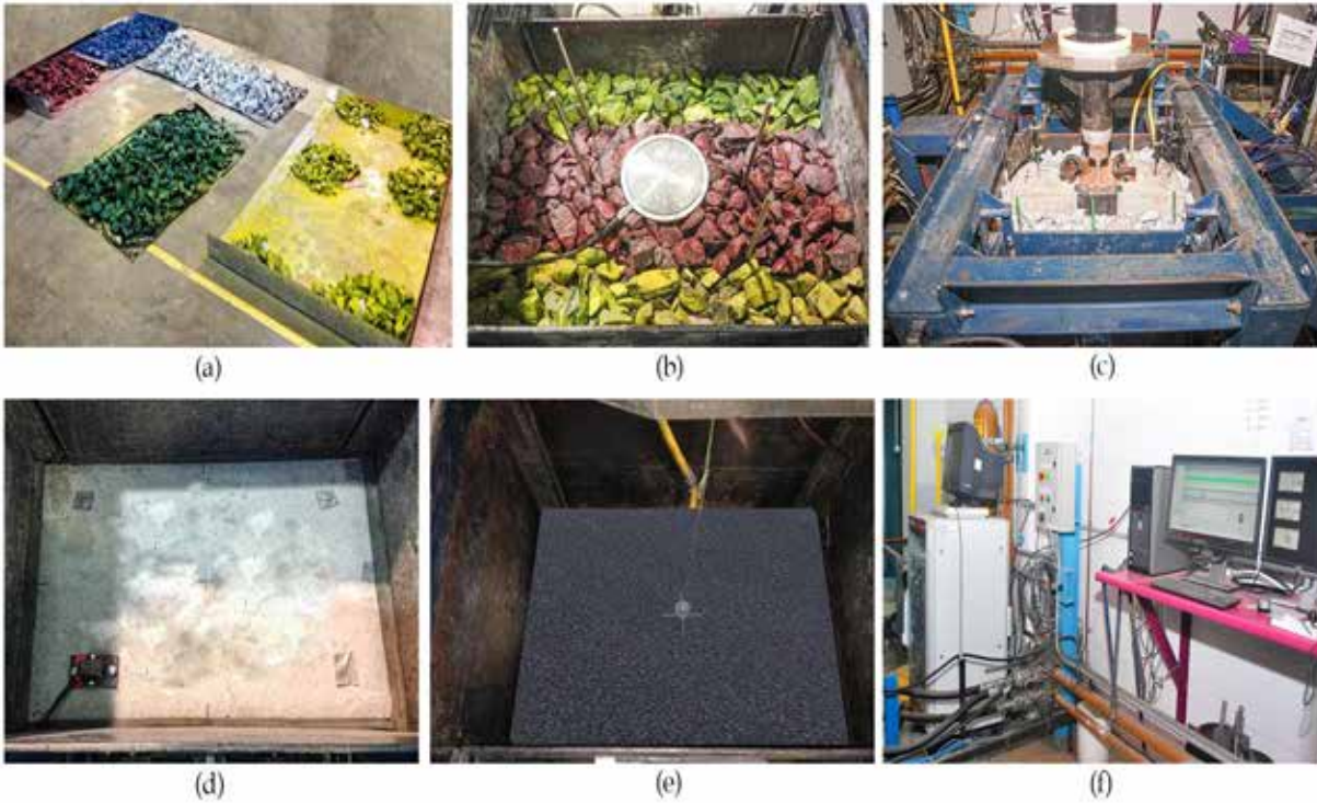
Figure 4 - (a) The ballast was colour coded to evaluate degradation with depth; (b) Coloured ballast layers compacted inside the triaxial chamber and instrumented with pressure cell and settlement plates; (c) Crib ballast filled around rail-sleeper assembly and potentiometers attached on top of the sleeper; (d) Concrete base is placed at the bottom of the triaxial chamber (e) UBM was placed on top of the concrete base; and (f) Load - frequency controller and data acquisition system.
