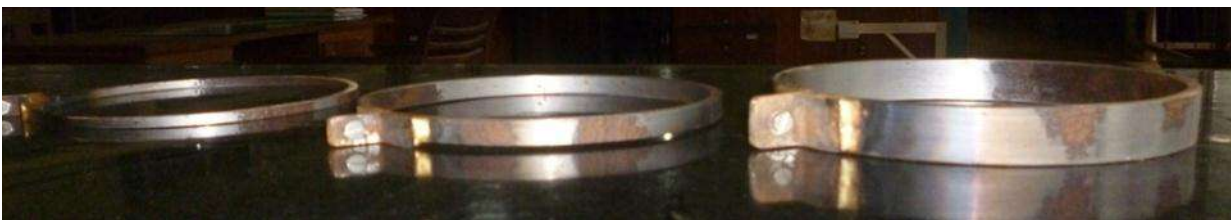
Figure 2 - Circular shaped templates to prepare specimens of thickness (i) 5 mm, (ii) 10 mm and (iii) 20 mm
