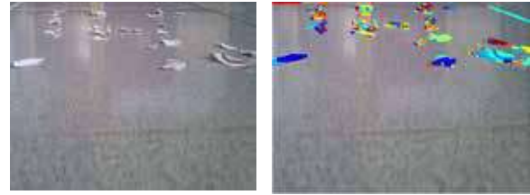
Figure 5-(a) Original dirt and (b) MSER dirt identified Feature
