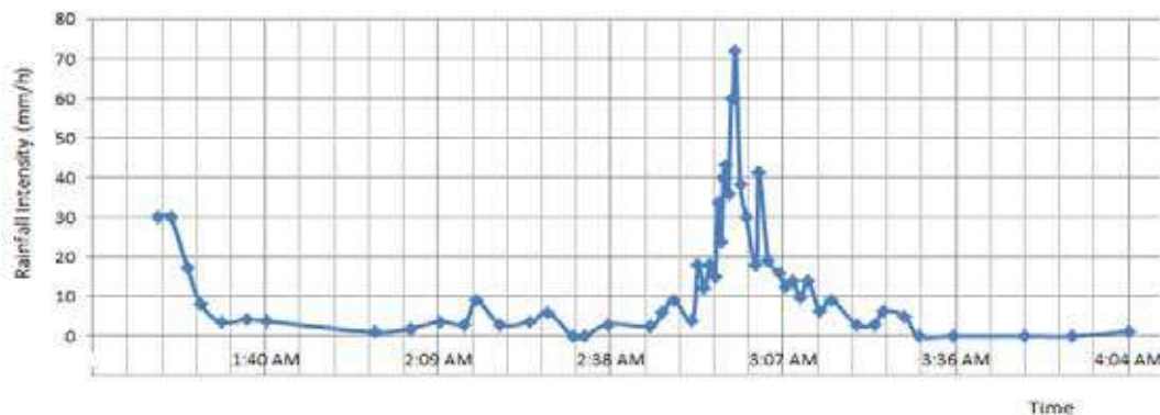
Figure 7 - Fluctuation in Rainfall Intensity (mm/h) Vs Time at Interstate Highway (I-275) Segment
