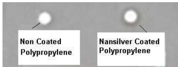
Figure 10 - Zone Inhibition of Non-coated Polypropylene and Nansilver Coated Polypropylene
