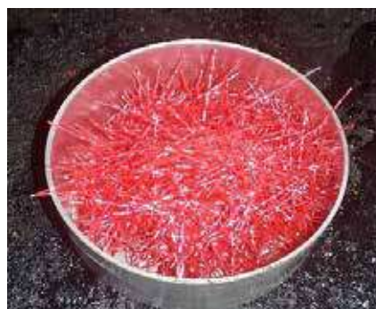
Figure 2 - Polyethylene Terephthalate (PET) of 0.5 mm, specific gravity 1.2 and melting
