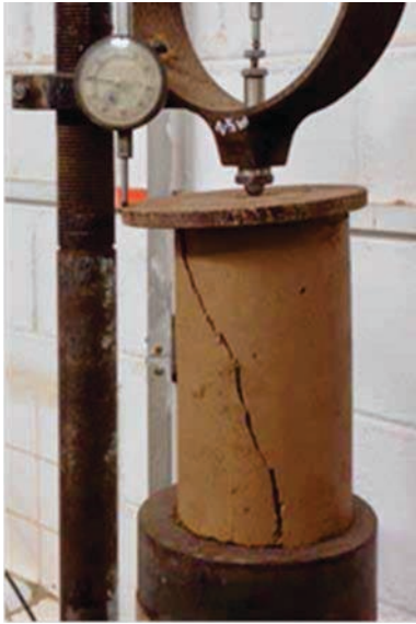
Figure 6 - Failure pattern for a sample
