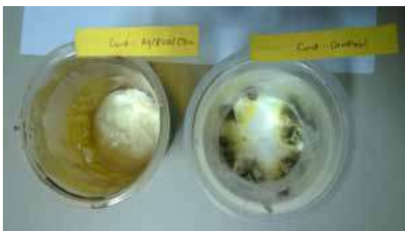
Figure 11 - Microorganism Growth of Non-coated Polypropylene and Nansilver Coated Polypropylene
